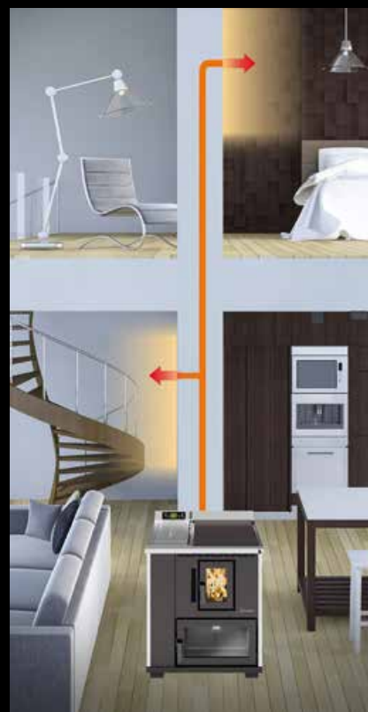
Canalization air chaud
